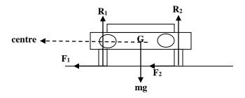
For no skidding, the centripetal force must be greater or equal to the centrifugal force i.e.
