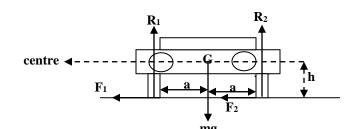
consider a vehicle with mass m moving with a speed v in a circle of radius r; let h be the height of the centre of gravity above the truck and 2a the distance between the tyres.
