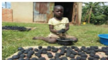
**Fig.14. Laying molded briquettes on a flat surface for drying.**
