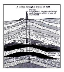
The drilling stem carries steel drilling pipes each 30ft long and 5 inches' diameter at the bottom is a powerful drilling bit that cuts its way through the earth and rocks.
